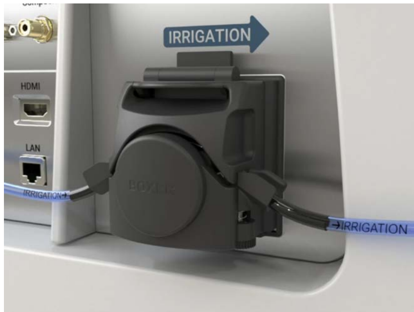
Figure 3.7 Irrigation Line Setup
