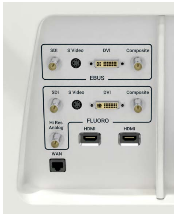
Figure 3.10 Audio Visual (AV) Connection Panel
