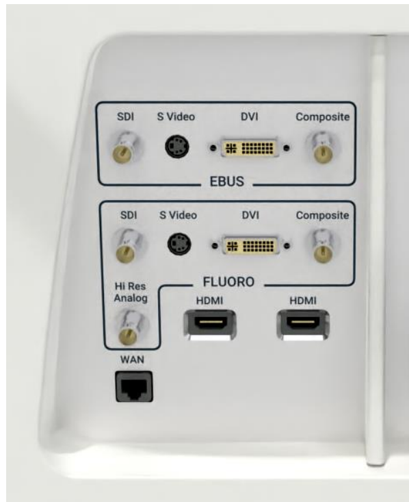
Figure 3.2 Audio Visual (AV) Connection Panel
