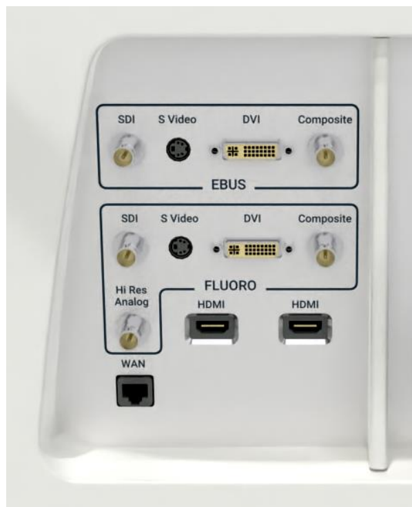
Figure 3.2 Audio Visual (AV) Connection Panel
