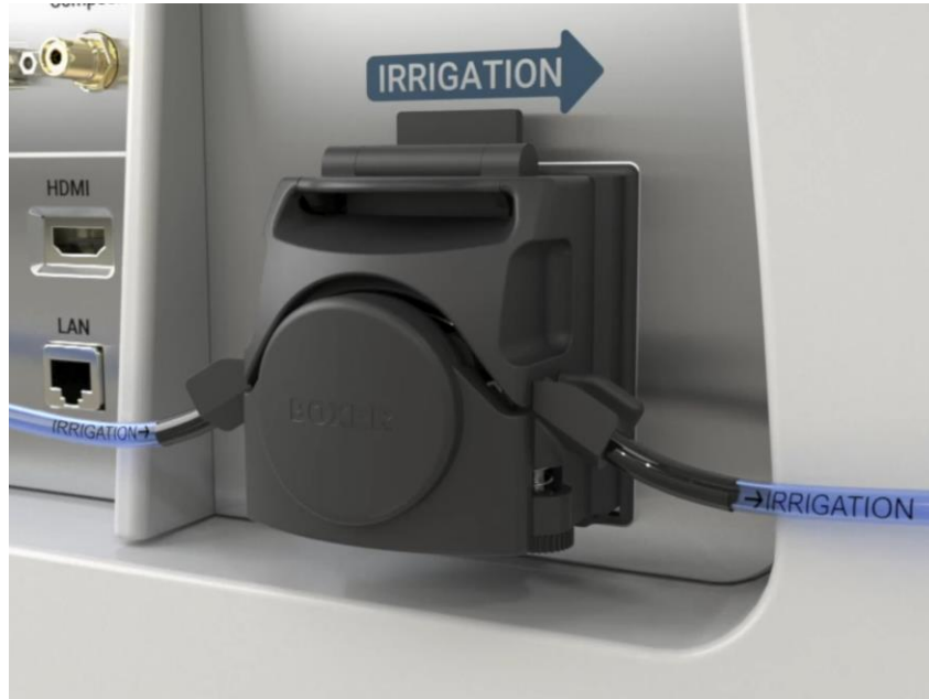
Figure 3.7 Irrigation Line Setup
