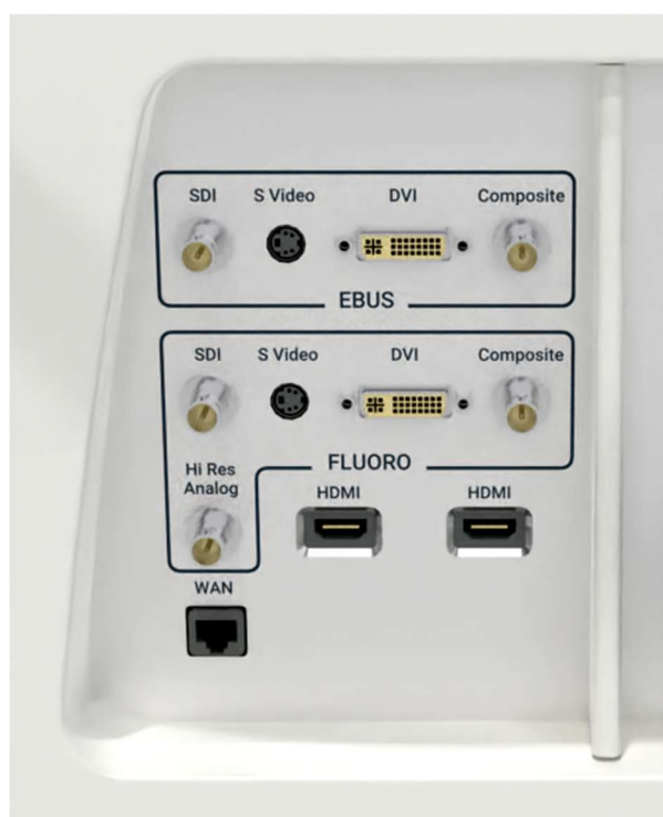
Figure 3.2 Audio Visual (AV) Connection Panel
