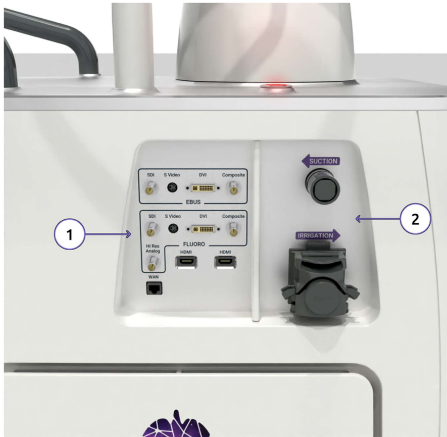
Figure 1.3 Audio Visual (AV) and Fluidics Panel
