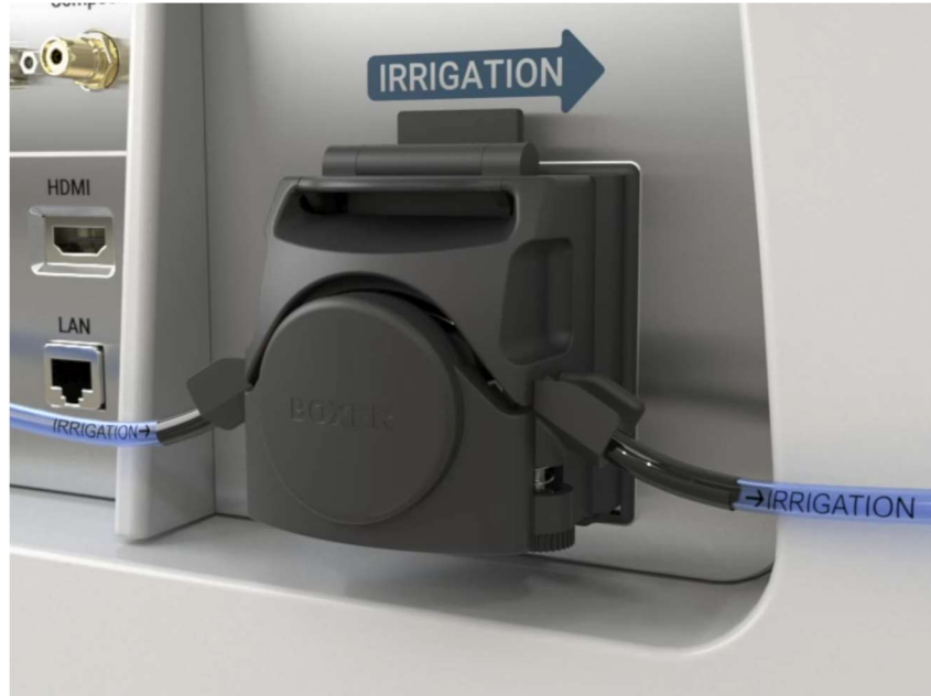
Figure 3.7 Irrigation Line Setup
