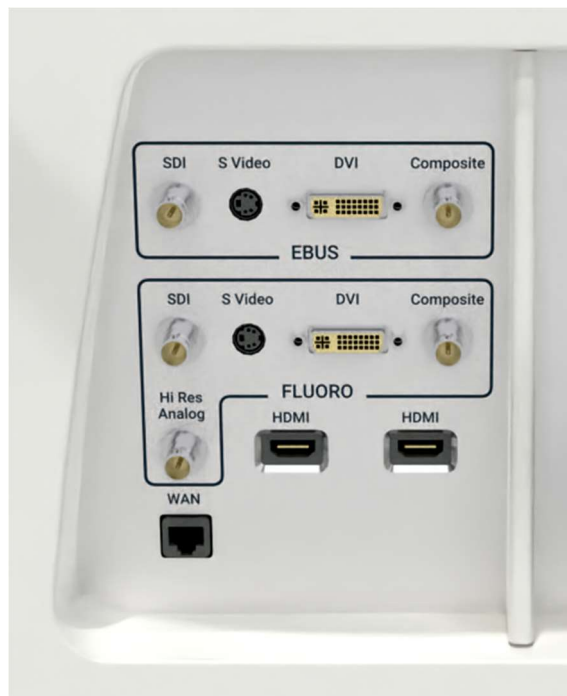
Figure 3.10 Audio Visual (AV) Connection Panel
